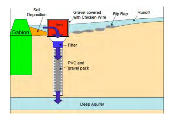
Figure 3. Example of filter: here the filter is placed right at the exit of the storm water drains, easily accessible. Source: Design of Recharge Well in the Dry Areas of Tunisia, Liz Hilkert, ABE-ENRE, 11 April 2005, Purdue University
