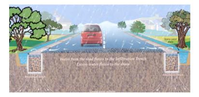
Here roads are built in such a way as to facilitate rainwater collection and ground water recharge through road-side trenches. They are about 600mm wide and 600mm depth, filled with pebbles /aggregates with a top layer of coarse sand. <u>Figure 3</u>. Schematic installation of the barrel system as rainwater collector for reuse or 'canalizator' of rainwater for aquifer resplenishment:
