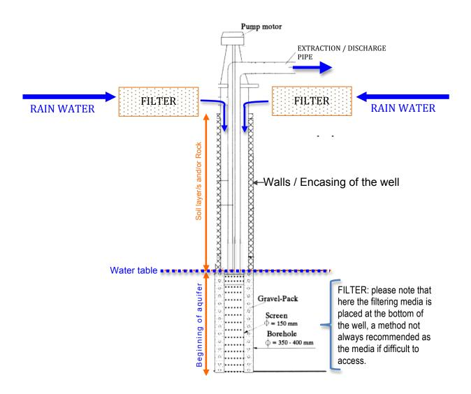
Figure 2. NOTE: Here 2 filters are being used between the water runoff and entrance into the aquifer, one with coarse gravel on top of the well, and another one below it, with finer particle media. Both structures are easy to access to change the filtering media. *Source: Design of Recharge Well in the Dry Areas of Tunisia, Liz Hilkert, ABE-ENRE, 11 April 2005, Purdue University*
